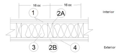
GYPSUM BOARD (Interior): Two layers USG Firecode<sup>®</sup> C Core, complying with ASTM C1396, min. 5/8 in. thick, 4 ft. wide applied vertically, fastened to framing. Face layer joints staggered with base layer and covered with paper tape and joint compound.
