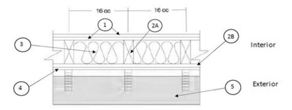
GYPSUM BOARD (Interior): Two layers Type X complying with ASTM C1396 min. 5/8 in. thick, 4 ft. wide applied vertically, fastened to framing. Face layer joints staggered with base layer and covered with paper tape and joint compound.
