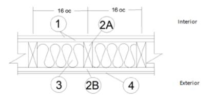
GYPSUM BOARD (Interior): Two layers USG Firecode<sup>®</sup> C Core, complying with ASTM C1396, min. 5/8 in. thick, 4 ft. wide applied vertically, fastened to framing. Face layer joints staggered with base layer and covered with paper tape and joint compound.
